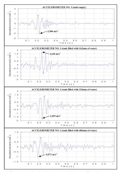
Fig. 5. Acceleration time histories under the Polkowice 2001 mining tremor (accelerometer no. 3)
